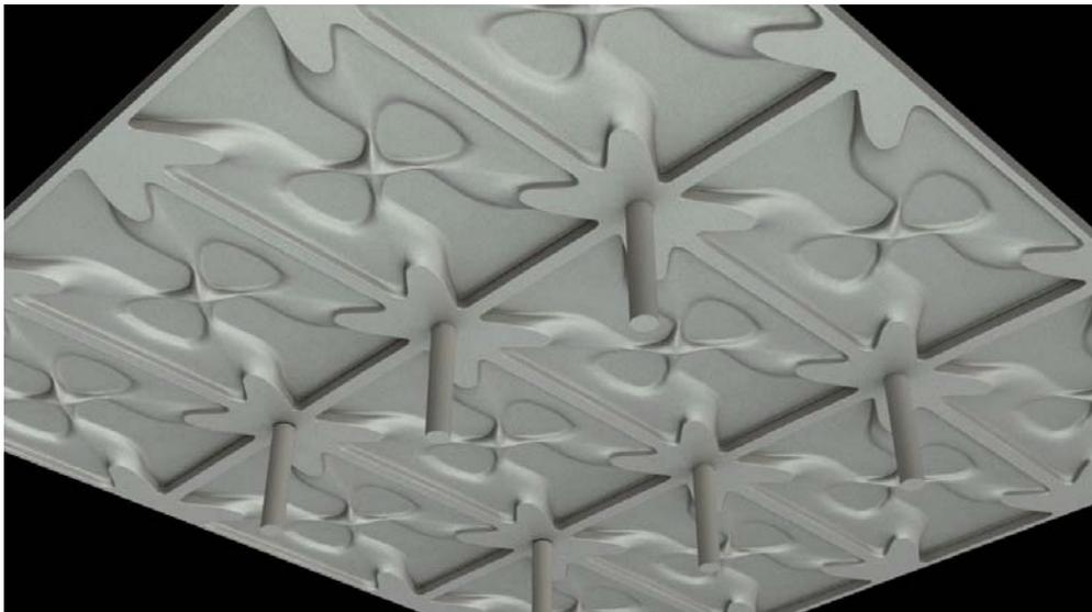
Figure 13: Computer rendering of loft structure of second revised optimisation result
